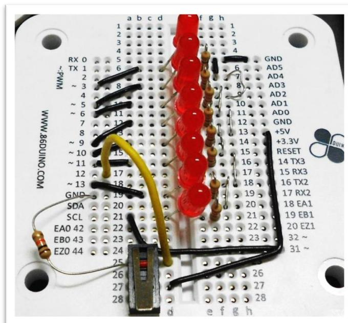
Fig-14: EduCake with LEDs, resistors and push button attached
