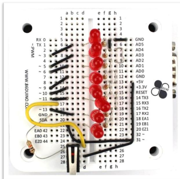
Fig-12: EduCake with LEDs and resistors attached – back view
