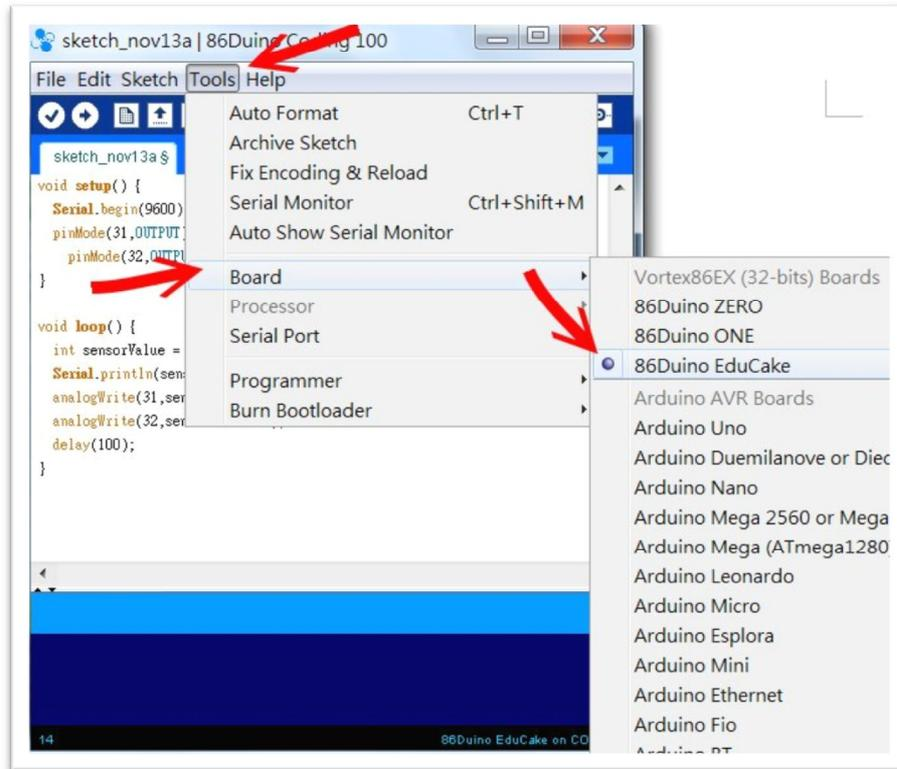
Fig-8: 86Duino IDE – Selecting target device
