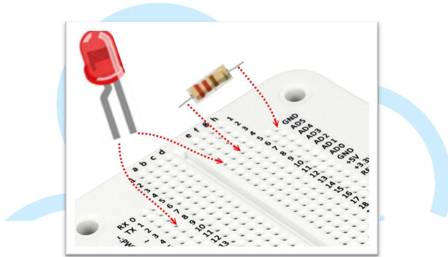
Fig-11: LED and resistor connected to the breadboard on EduCake
