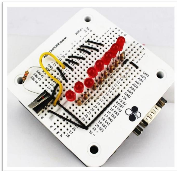
Fig-13: EduCake with eight LEDs and resistors attached – Front view
