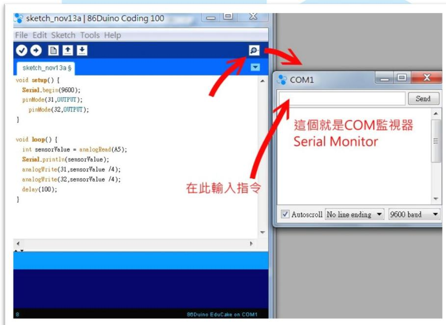
Fig-15: Serial Monitor - sending command to turn on LED
