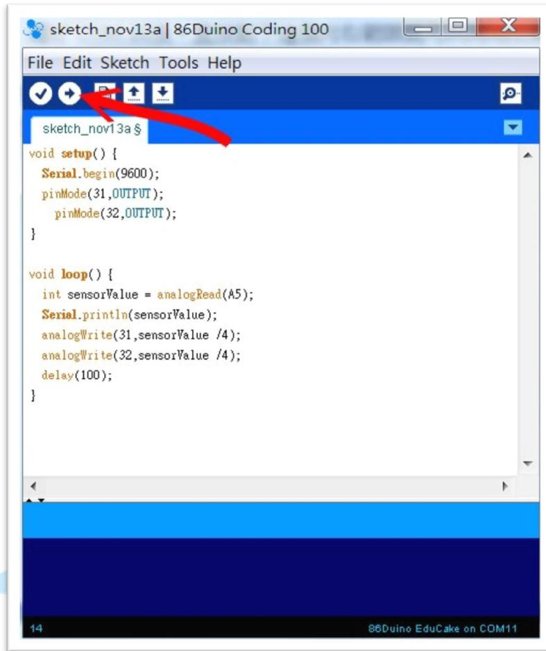
Fig-10: 86Duino IDE – Deploy application to target device
