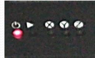
3. all LED on the panel lights blink once after leaving Red lighted.
