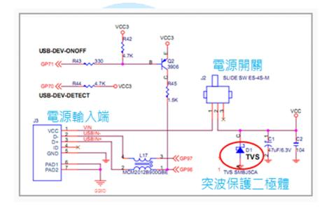
While the EduCake is using a simple power circuitry, from the above schematic, you can see the circuit includes surge protection to protect the internal circuit against power surge during initial power on.
