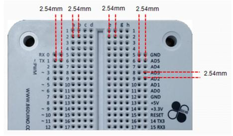
The following figure shows the connectivity for the pins on the solderless breadboard, where each yellow-line marks the pins that are connected (shorted):
