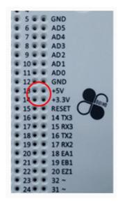
To prevent damage to the EduCake's internal component caused by over current through the 5V and 3.3V output pins, there is a 1.0A fuse added to each of these 2 pins, as shown in the figure below:
